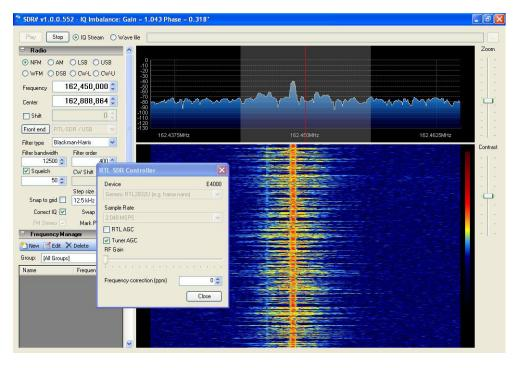
In the next step we us the up/down arrows to adjust the ppm correction to bring the tuning indicator to the center of the signal carrier. In the above example, the receive mode is NFM (narrow FM), and the center of the carrier is plainly visible.
