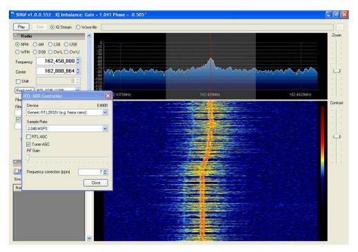
The carrier center is below the expected position on the display, so we will use the up arrow to add the ppm multiplier to the signal. If the carrier center was higher than the expected position (on the tuning indicator), we would use a negative adjustment.
