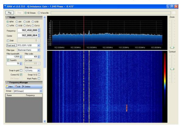
You will notice that the tuning indicator is located directly on the peak at that location indicating a properly tuned dongle. To achieve this there are only a few simple steps involved. Without any ppm adjustment (set to 0), the display may look more like the one below.
