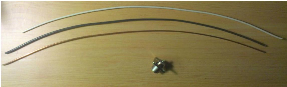
Strip the outer sleeve from the romex and you'll have an unshielded ground wire, and white and black insulated wires. Strip these so that you end up with three bare copper wires.
