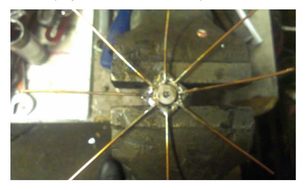
Finally take the last wire and solder it into the center piece of the SO-239.
