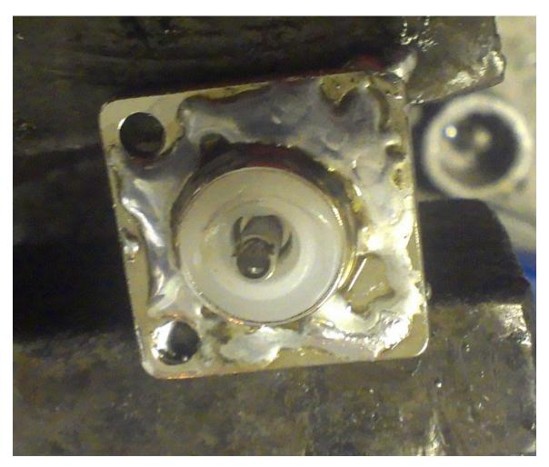
Next apply some solder to one end of each of the lengths of wire. WARNING: use the pliers to hold the wire while doing this. Copper is and extremely good conductor of heat, and you will burn yourself if you don't.
