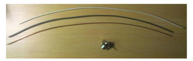
Strip the outer sleeve from the romex and you'll have an unshielded ground wire, and white and black insulated wires. Strip these so that you end up with three bare copper wires.
